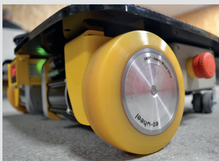
SWD ® Core Safety gear motor with 125 mm castors
