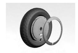
Remove the tyre and the inner tube.
